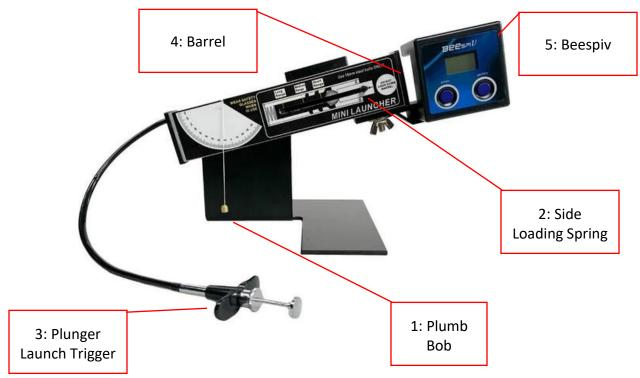
Today you'll be working with the above shown mini projectile launcher with detachable speed measurement device.
