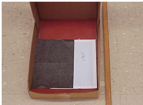
Figure 9 - Setup showing how to measure the horizontal reference distance D_r using masking tape on the floor. Fine cell graph paper is taped on the rubber mat in a cardboard box lid. Carbon paper placed face down on the graph paper leaves black impression marks where the steel ball lands.
