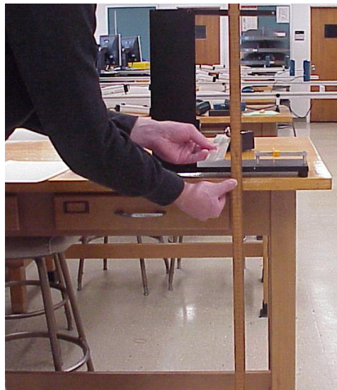
Figure 8 - Measuring method to determine H using a 2 meter stick and small ruler placed under the steel ball and held horizontally. The other end of the vertical 2 meter stick is on the ground.
