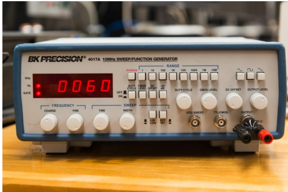
Figure 3: Our BK precision Function Generator will be used to generate signals to test our electrical circuits we make in future labs. Different waveforms behave uniquely in different circuits, so it is important we know how to create a variety of signals.
