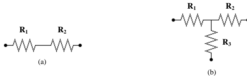
FIGURE 1 - Circuit diagrams. (a) R_1 and R_2 are in series. (b) R_1 and R_2 are not in series.
