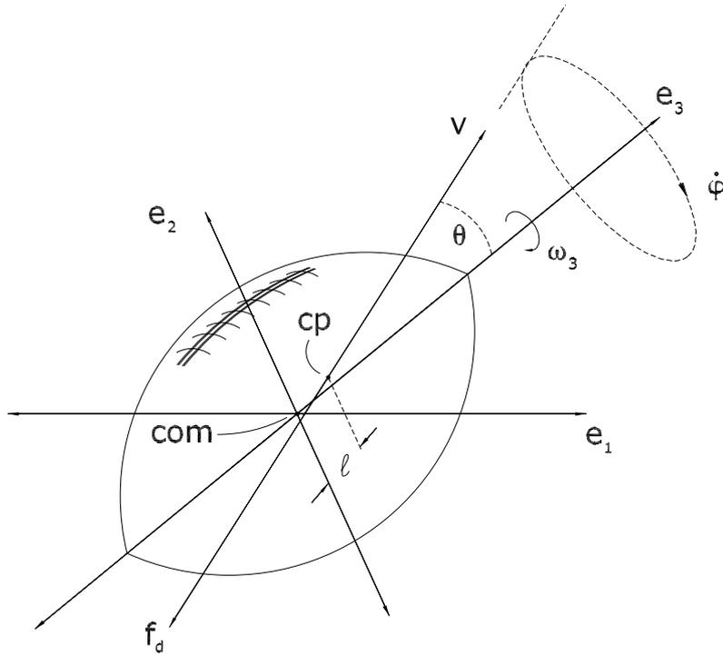
FIG. 2: Center of mass, center of pressure (CP), velocity and drag force on the ball. The drag force  $f_d$  acts along the velocity direction and through the CP. We take  $\theta$  as the angle between the force and the  $e_3$  axis. The aerodynamic torque is then  $\tau = f_d l \sin \theta$ .
