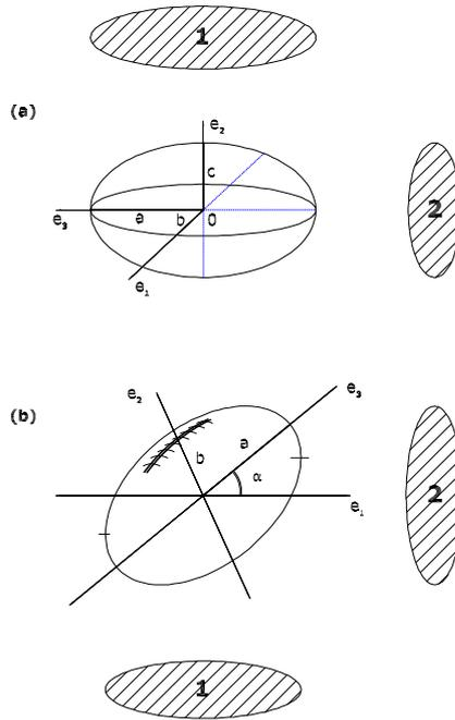
FIG. 4: The surface area the football presents, at different inclination angles in flight. Fig 4(a) show maximum surface area  $\pi ab$  vertically and minimum surface area  $\pi b^2$  horizontally. Fig. 4(b) has an inclination of  $\alpha$  and the surface area this football presents to the vertical and horizontal has changed.
