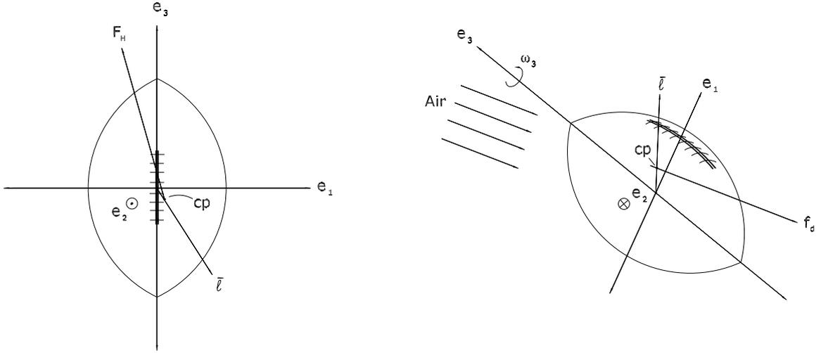
FIG. 3: This figure shows the initial throw and the position of the CP towards the hand, and the CP in flight when it shifts forward. The torque directions are also shown as  $e_2$ . We assume the football is thrown by a right handed player. First it yaws left and then right. The overall motion is slightly to the right for a right handed player.
