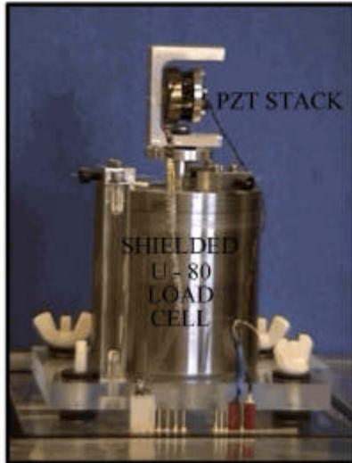
FIGURE 2: The PZT stack mounted on the U-80 load cell.
